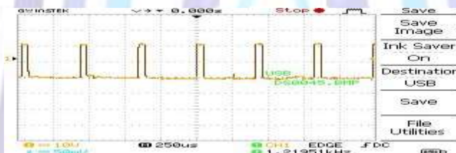
Figure .15. Gate Pulse to Rectifier Switch S2
