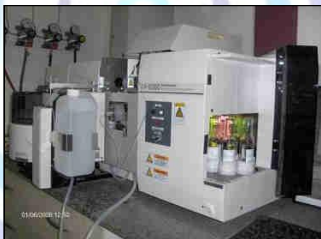
Fig. 10 – Atomic absorption spectrophotometry equipment with electrothermal atomization
