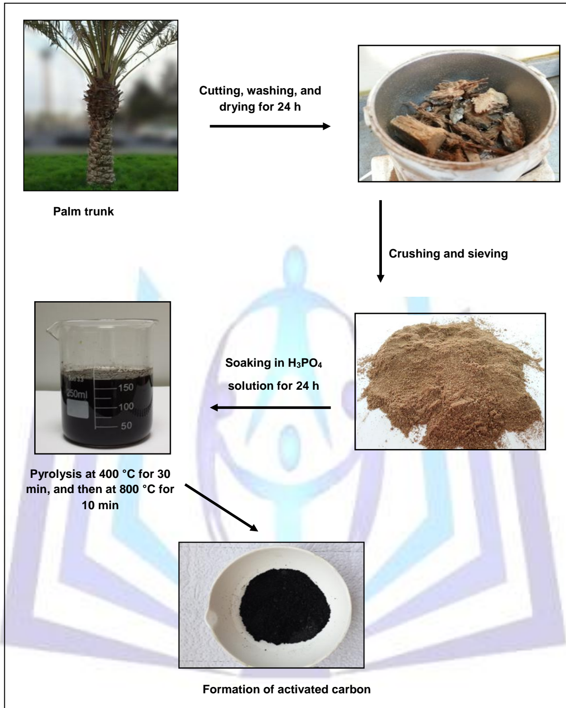
Fig 1: The process carried out on fabrication of activated carbon from date palm trunks.
