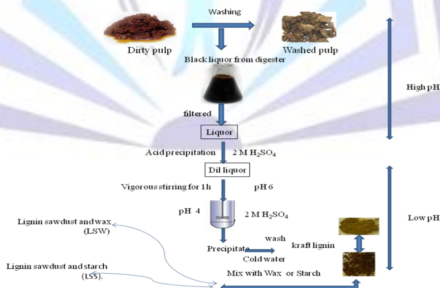
Fig. 1. Schematic diagram for lignin separation and preparation of the biocomposites.
