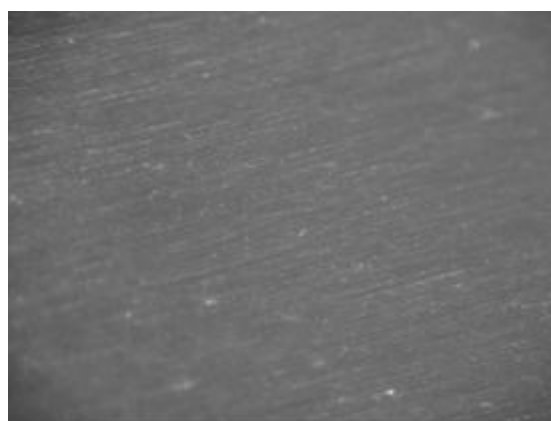
Fig. 11. Optical micrograph of Al electrode surface after potentiodynamic polarization in 0.5 \text{ mol dm}^{-3} NaCl solution with addition green tea extract
