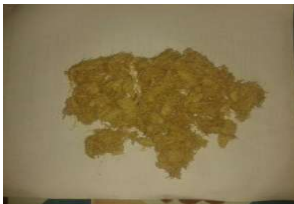
Fig 2 Obtained Treated Cellulose from Cross and Bevan method
