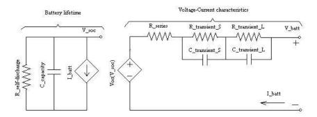
Fig 10: Model of Lithium-ion Battery
