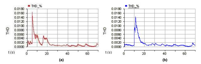
Fig 14: Voltage total harmonic distortion (THD<sub>v</sub>) plots with (a) vanadium redox battery and (b) lithium-ion battery
