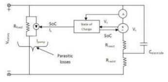
Fig 7: Model of Vanadium Redox Battery
