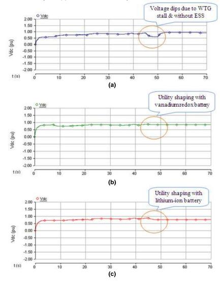
Fig 13: DC bus voltage shaping for intermittent wind power from 45s to 50s (a) without energy storage, (b) with vanadium redox battery energy storage and (c) lithium-ion battery energy storage
