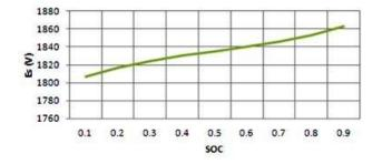
Fig 6: Lithium-ion battery 500 cell stack voltage for varying SOC
