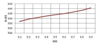
Fig 5: Vanadium redox battery 500 cell stack voltage for varying SOC
