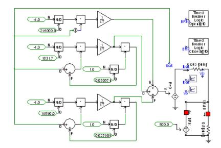
Fig 11: PSCAD model of lithium-ion battery with charge (800 A), until 15s and discharge (0.8Ω), for next consequent 25s
