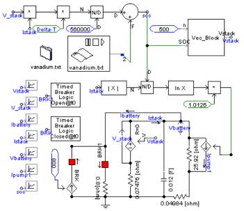
Fig 8: PSCAD model of VRB with charge (800 A), until 60s and discharge (0.8Ω), for next consequent 60s
