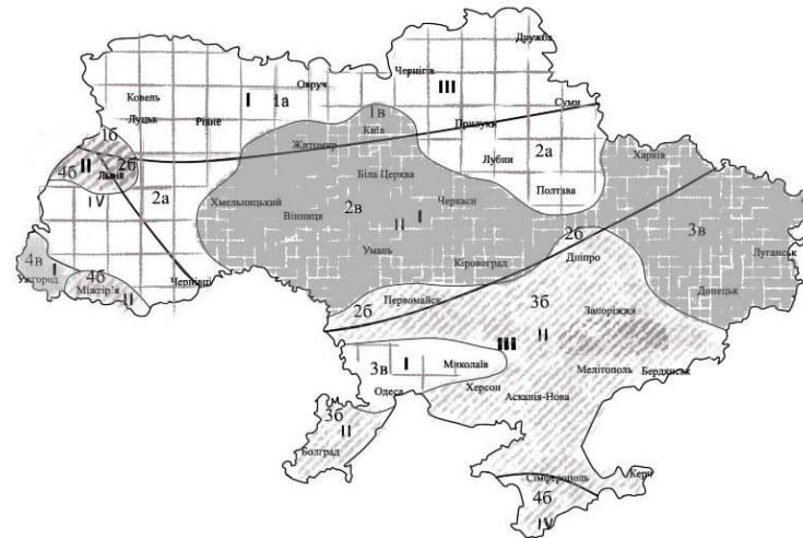
Fig. 4. Map of road-climatic zoning of the Ukraine territory by average rainfall indicators
