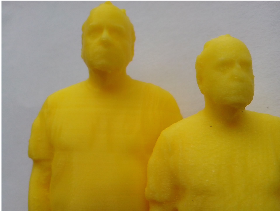
Figure 5.10: 3D printed model with low level-of-detail (right)
