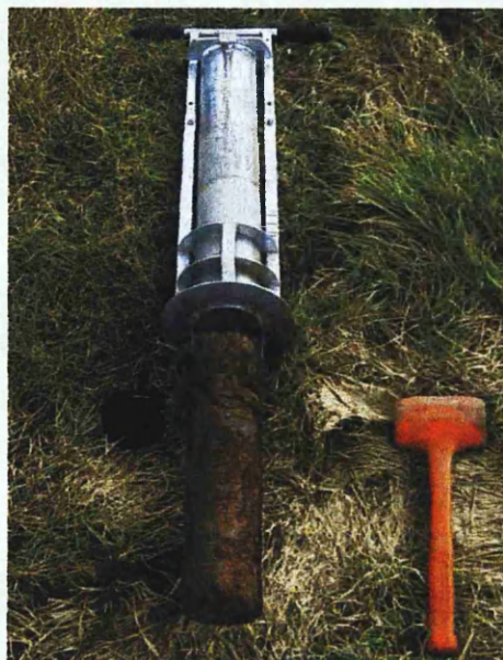
Figure 4.4. Golf hole corer used throughout the project to obtain soil cores.
