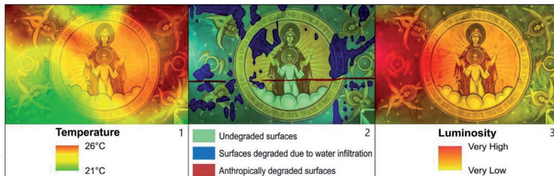
Figure 5. Distribution of temperature, luminosity and degraded areas on the painting on canvas “Virgin Mary with the Baby Jesus” (after Oana et al., see [42]): (1). Temperature distribution at the canvas level; (2). Distribution of degraded areas at the canvas level; (3). Distribution of natural light at the canvas level.
