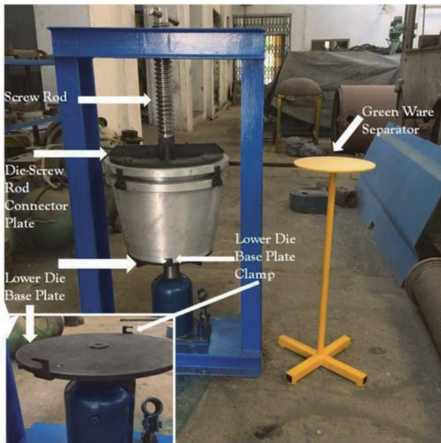
Figure 4. Filter press operated with screw and hydraulic system [11].
