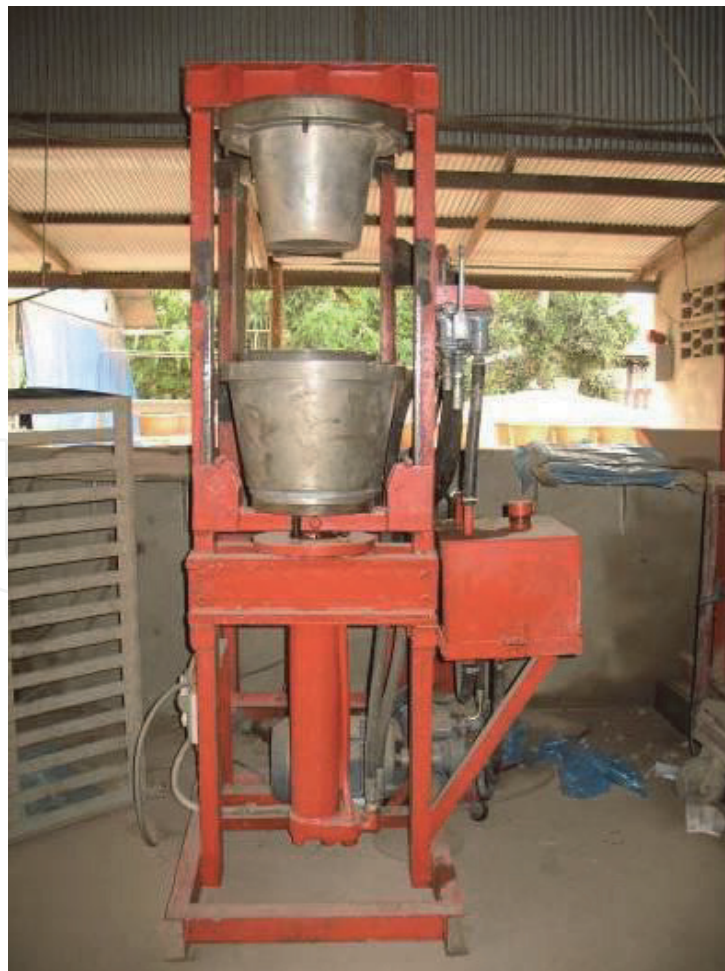
Figure 7. An electric motor driven hydraulic press [12].
