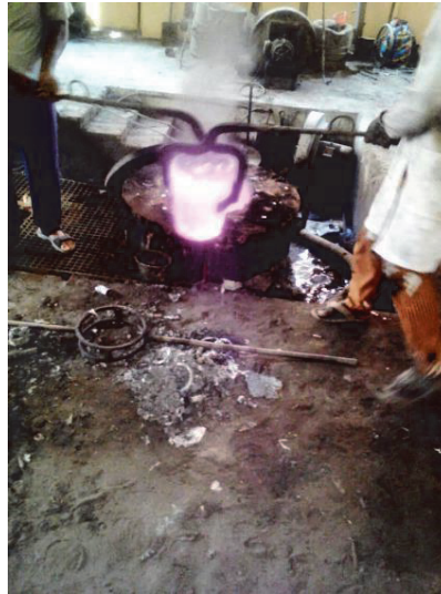
Figure 16. Removing molten aluminium from the furnace using a pair of tongs.
