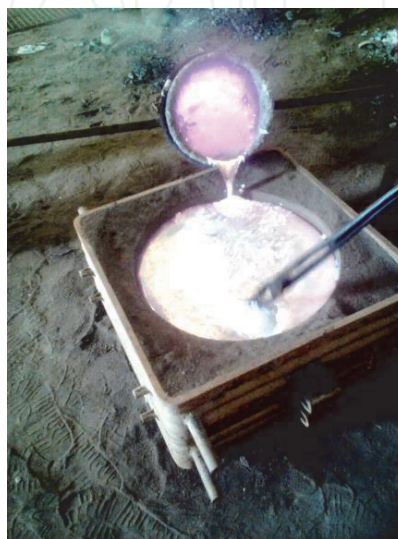
Figure 21. Poking the poured-in metal to remove trapped air.
