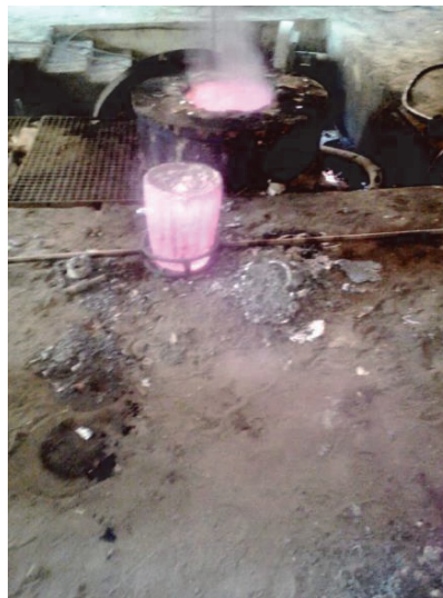
Figure 17. Crucible set in the carrier rod in readiness for casting.
