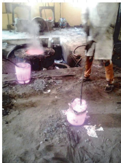
Figure 18. Stoking the molten metal to remove dross and other particles.
