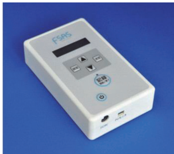
Figure 16. Compact F-SAS sensor system (175 × 100 × 45 mm, 390 g, voltaic drive during electric outage) (after improvement).
