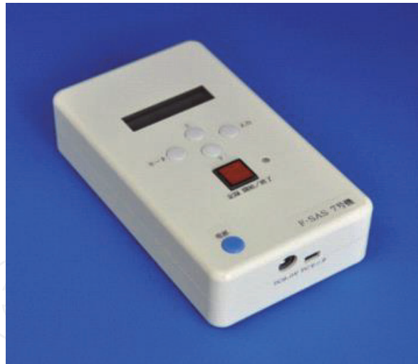
Figure 15. Compact F-SAS sensor system (175 × 100 × 45 mm, 390 g, voltaic drive during electric outage) (before improvement).
