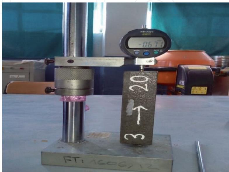
Figure 14. Shrinkage measurement on prismatic test piece.
