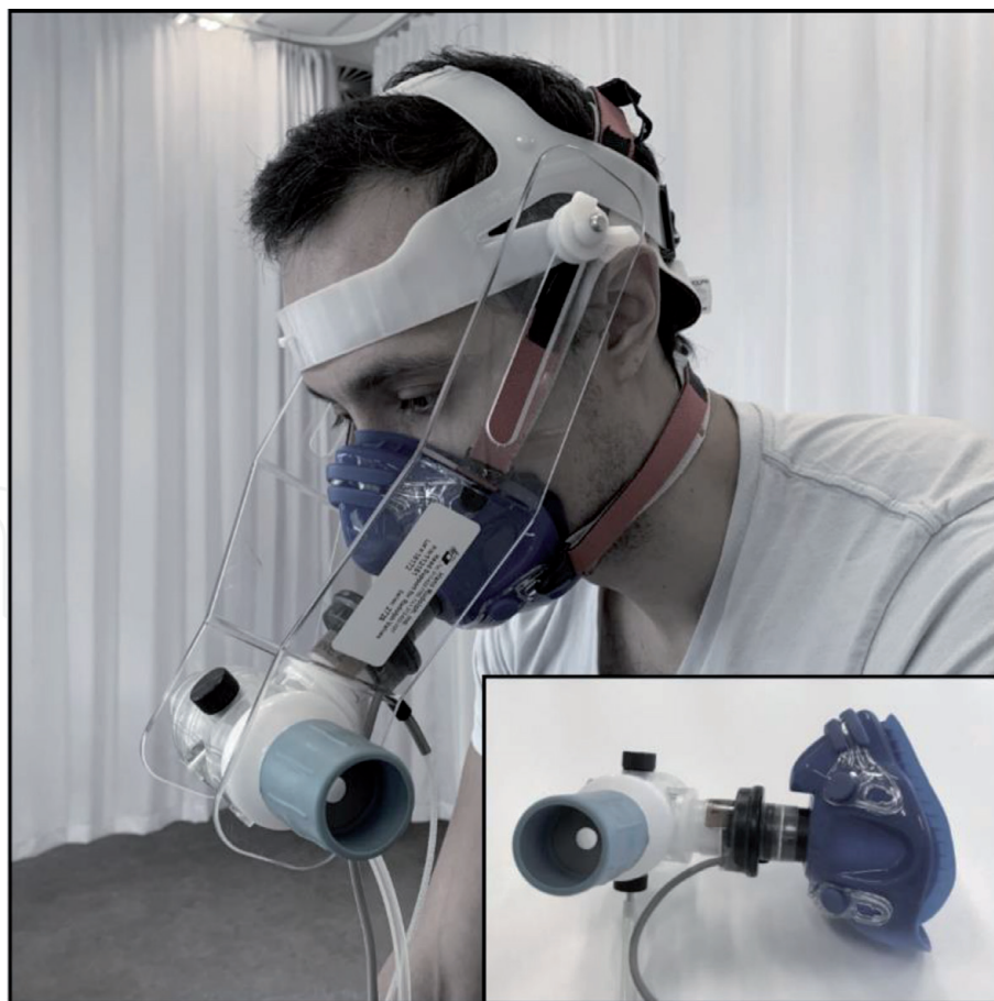
Figure 1. Representation of how inspiratory loading was achieved [62]. A plastic disk with a 10-mm opening was placed over the inspiratory side of a two-way non-rebreathing valve (Hans Rudolph Inc., Kansas, United States of America) attached to the distal end of a bidirectional turbine and held in place by the internal ridge of a rubber tubing adaptor. A pressure transducer was attached to the saliva port of the non-rebreathing valve via Tygon tubing to assess inspiratory mouth pressure.
