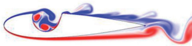
Figure 12. The vorticity contour plot over the airfoil with a cavity [63].
