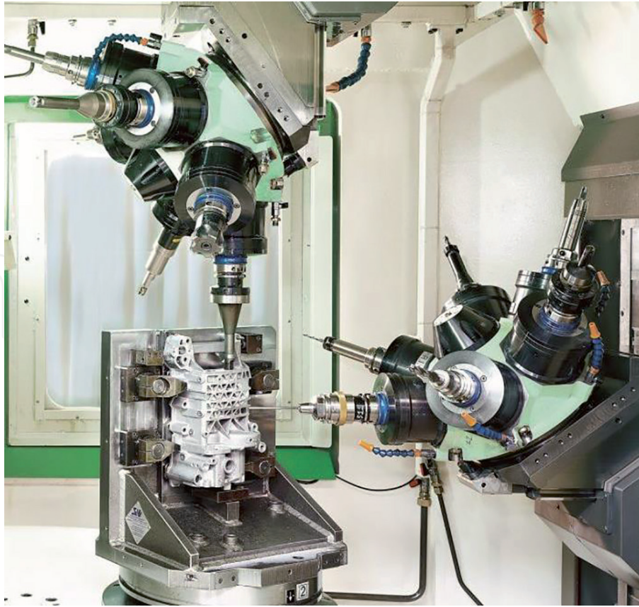
Figure 7. Concept 2, reconfiguration by adding new elements to the assembly (in production technology, spindle heads from Riello Sistemi).
