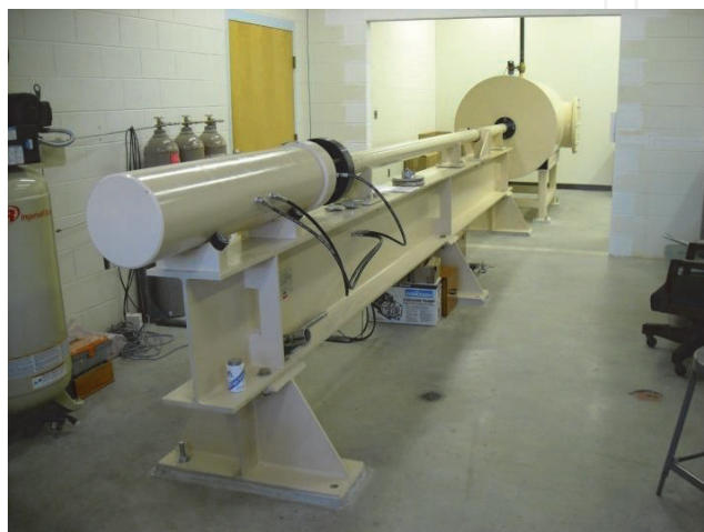
Figure 5. Gas operated facility for testing concrete samples.
