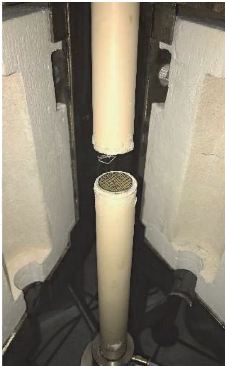
Figure 2. Image of the experimental equipment for the test of the solid oxide cells.
