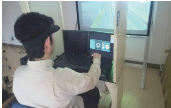
Figure 4. Experimental setup using train driving simulator [11].
