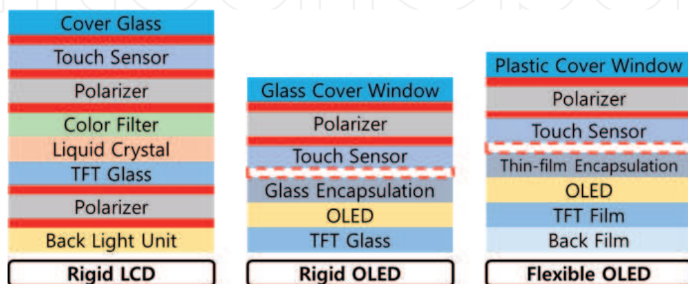
Figure 1. Multilayer structures of the display. OCA or PSA can be applied to red layers in the structures. A touch sensor can be placed on the encapsulation by OCA or direct deposition.
