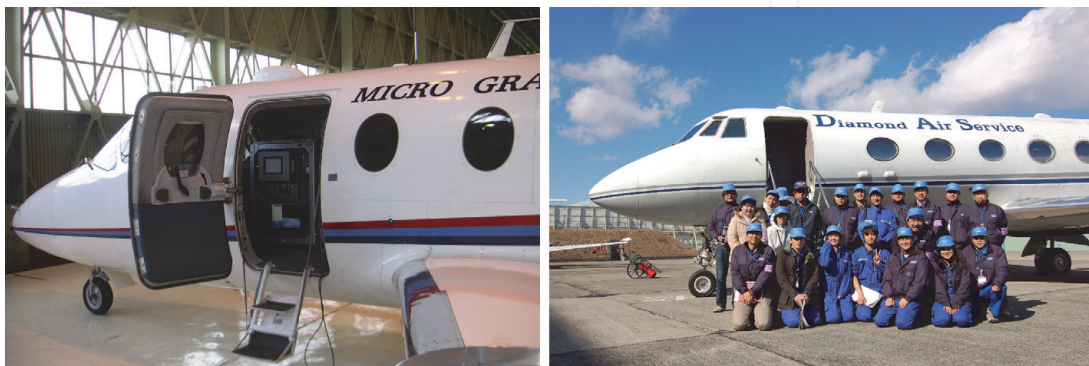
Figure 1. Aircrafts for parabolic flights operated by DAS. There are two types of the aircrafts. One is MU-300 from Mitsubishi heavy industries loading two racks (left), and the other is G-II from Grumman aircraft engineering Corp. For four racks (right).
