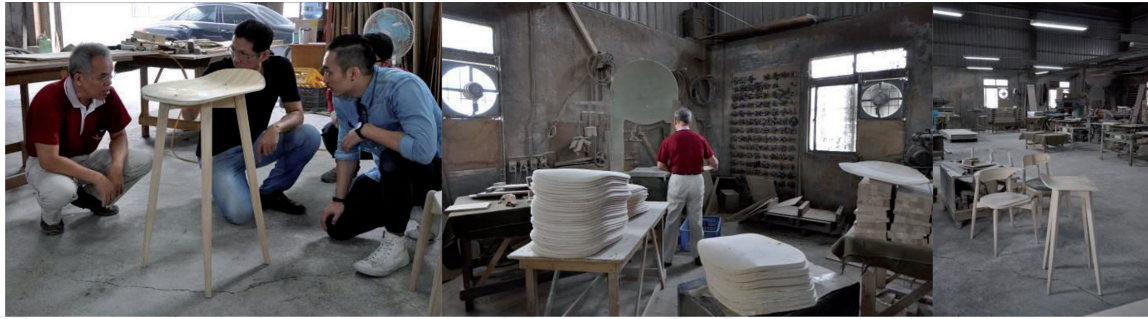
Figure 1. In the sampling process, the designers and sample makers need repeated discussions and corrections to understand the exact proportion and shape of furniture.
