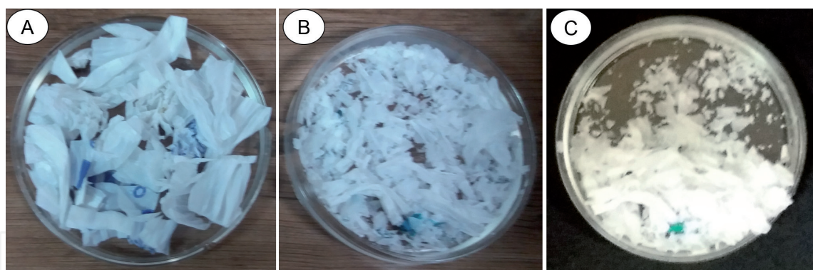
Figure 3. Oxo-biodegradable plastic bags before (A) and after 21 months of exposure to sunlight (B and C). The letter C shows the fragmented plastic.
