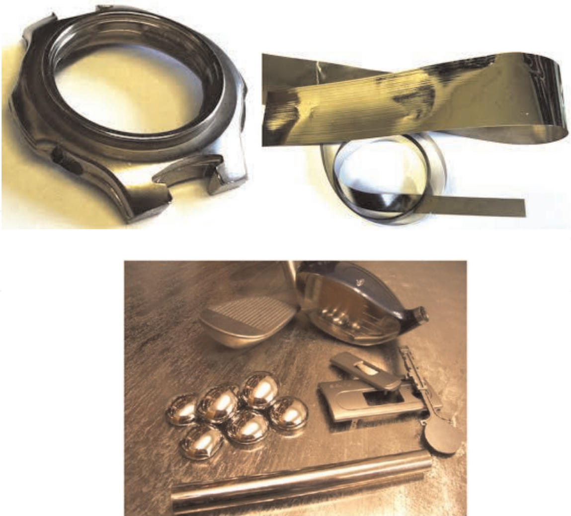
Figure 6. BMG articles fabricated by direct casting method.
