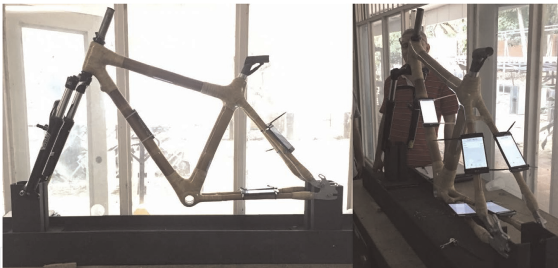
Figure 10. Setup of modal test.
