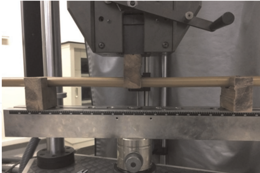
Figure 4. Setup of three-point bending test.
