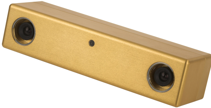
Figure 3.3: Bumblebee 2 - Point Gray Research stereo camera.
