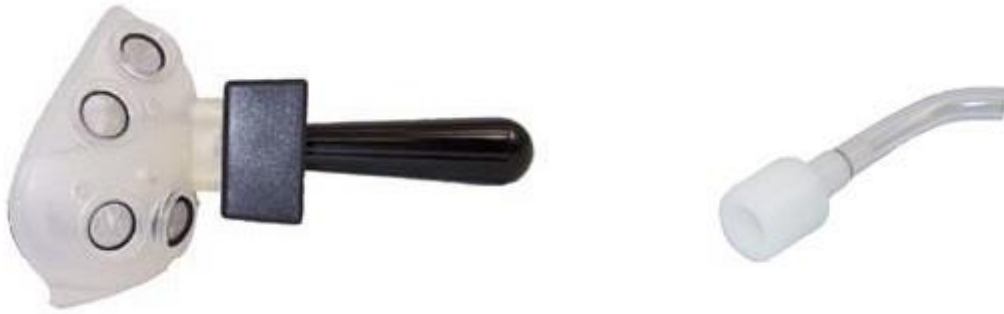
Figure 9. Rothenberg mask (in the left), used for measuring oral flow and intra-oral pressure pressure transducer (in the right) (adapted from www.glottal.com/ , consulted in 10-01-2014).
