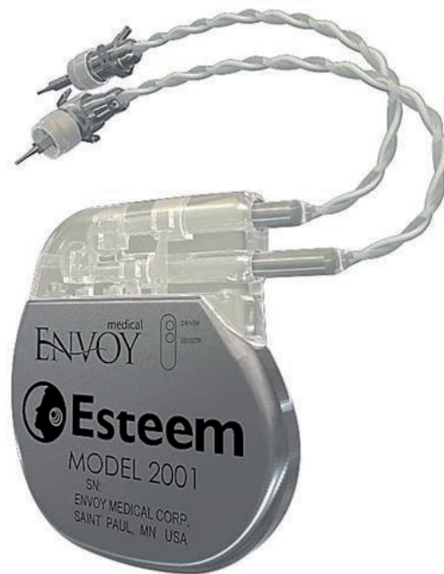
Figure 1. The Esteem ® middle ear implant. The sound processor is connected to the two transducers, namely the sensor and the driver.
