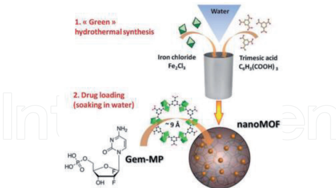
Figure 2. Representation of Gem-MP encapsulation into MIL-100(Fe) [3].
