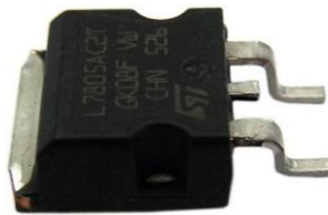
Figure 32: L7805 used as 5V voltage regulator in the TURF system [51]
