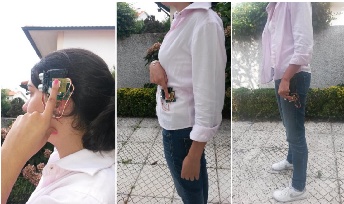
Figure 44: Testing positions of the TURF system: Head (Left), Body (Center), Leg (Left)
