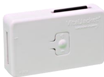
Figure 15: VitalJacket® box Digital Recorder [3]
