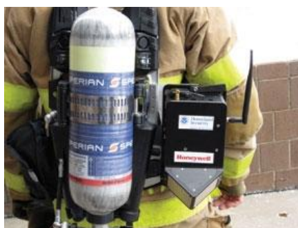
Figure 13: GLANSER implemented on fireman's suit [31]
