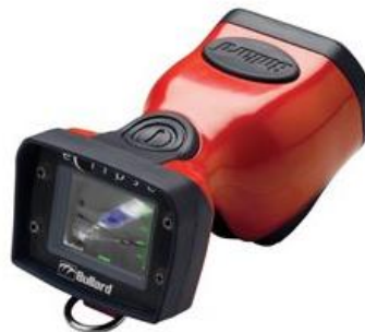
Figure 8: Thermal Camera for firefighting use [21]
