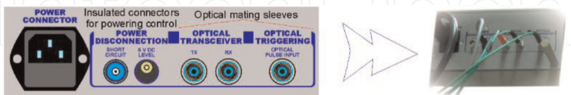
Figure 4. Elements of mobile measuring stands used for powering management and optical communication [19].
