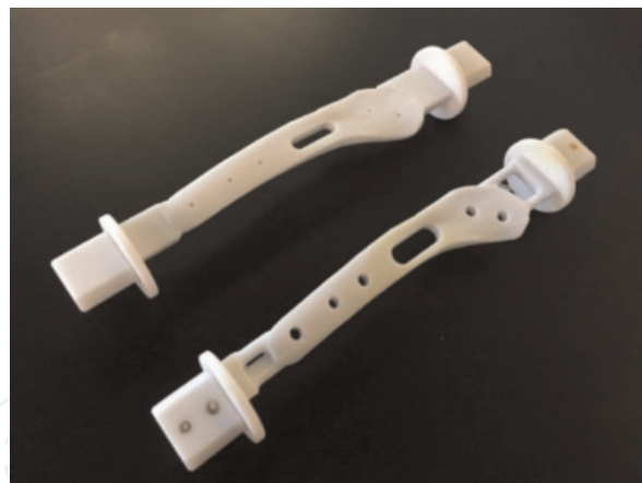
Figure 11. Case study of using FAH-PS for finishing of a patient-specific bone plate (reproduced with permission from [16]).
