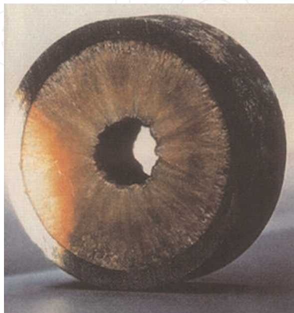
Figure 1. Sectional view of pipeline affected with acute wax deposition [14].
