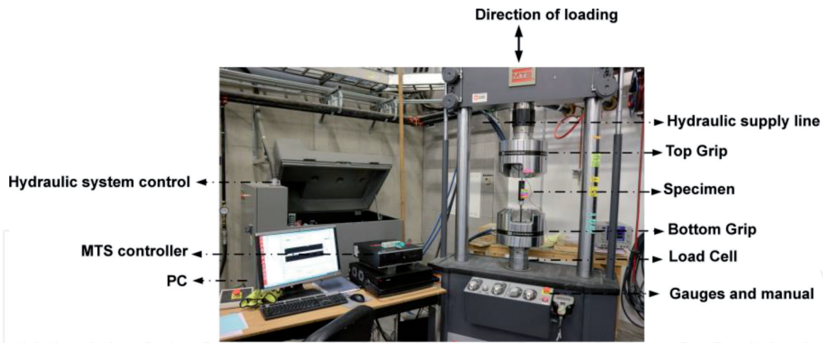
Figure 2. The MTS loading frame machine and its accessories.
