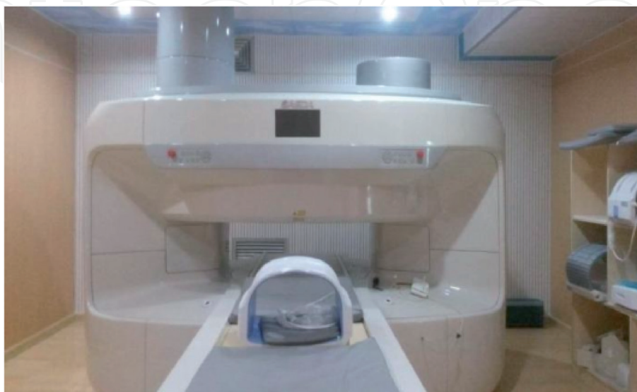
Figure 1. A 0.7 T whole-body open MRI system.
