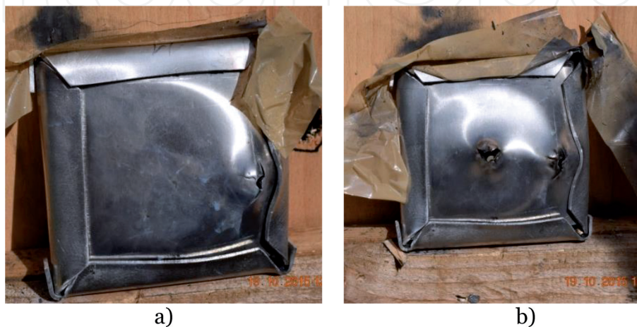
Figure 17. HEA-steel ballistic package during dynamic tests (a) after the first firing and (b) after the second firing.
