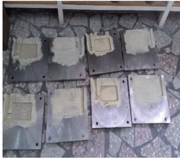
Figure 2. Metallic molds for casting Al_{0.8}CrFeCoNi alloy.
