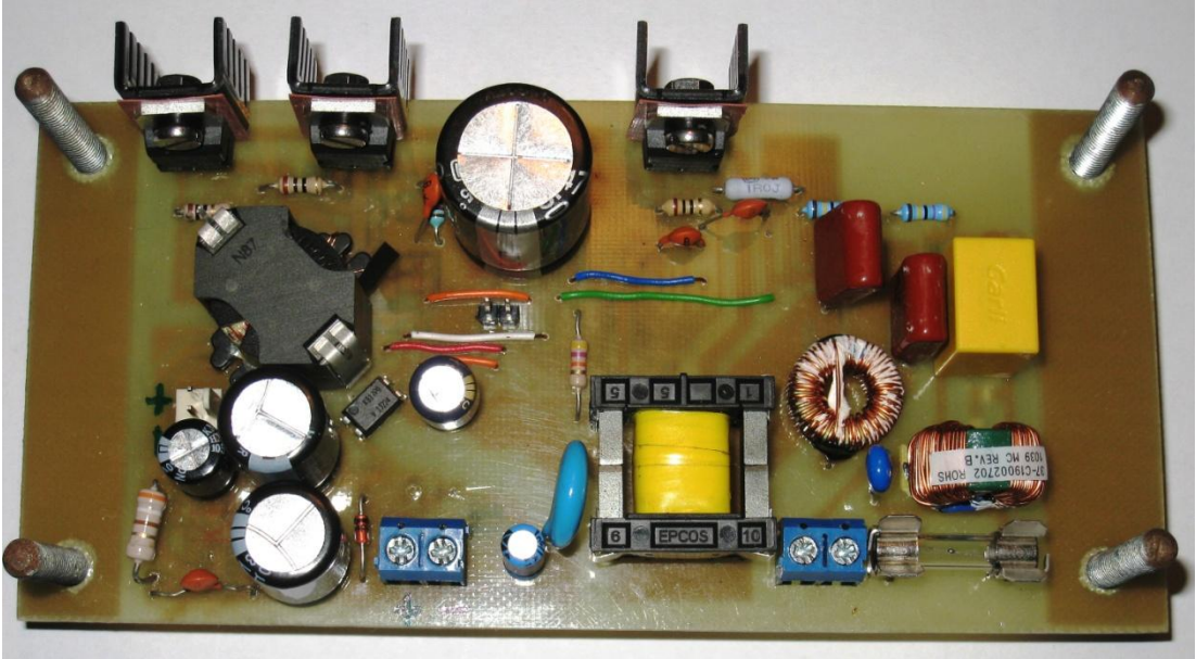
Figure 4.2 Photograph of Power supply board.
