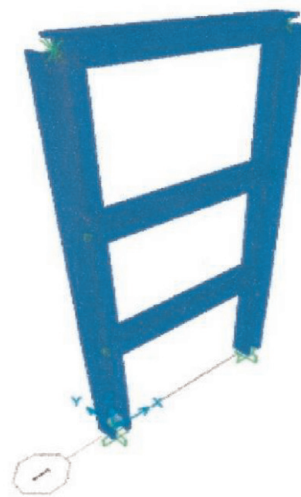
Figure 4. Numerical model made in SAP2000 ® structural analysis software, with position of loads and their magnitudes.
