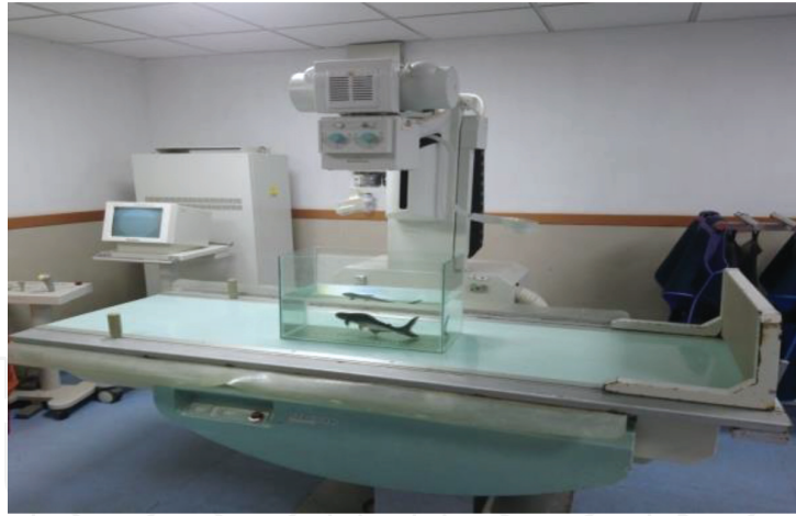
Figure 14. Digital fluoroscopy recording of fish swimming.
