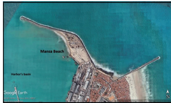
Figure 3. The residual bypass of sand across the jetties and the headland created the Mansa Beach and keep nourishing it regularly. The bypass also produces the silting of the harbor's basin, which has to be frequently dredged.
