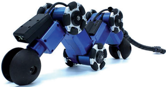
Figure 7. A multi-link-articulated wheeled-type in-pipe robot named AIRo-2.2 [20].
