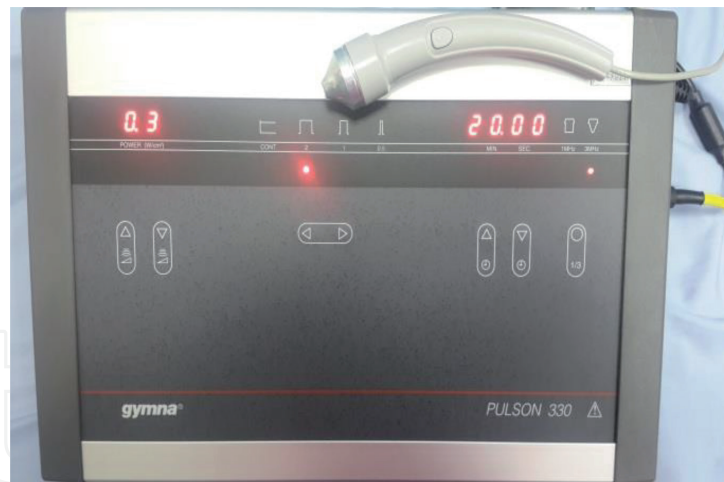
Figure 2. The therapeutic ultrasound machine Gymna Pulson® 330 with intraoral probe and actual setting parameters on display.
