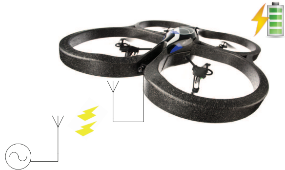
Fig. 1: Depiction of a drone charging with resort to microwave power transmission.
