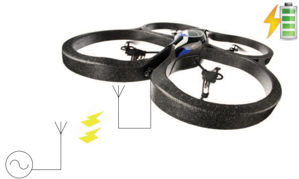
Fig. 2: Representation of a drone charging with resort to microwave power transmission.
