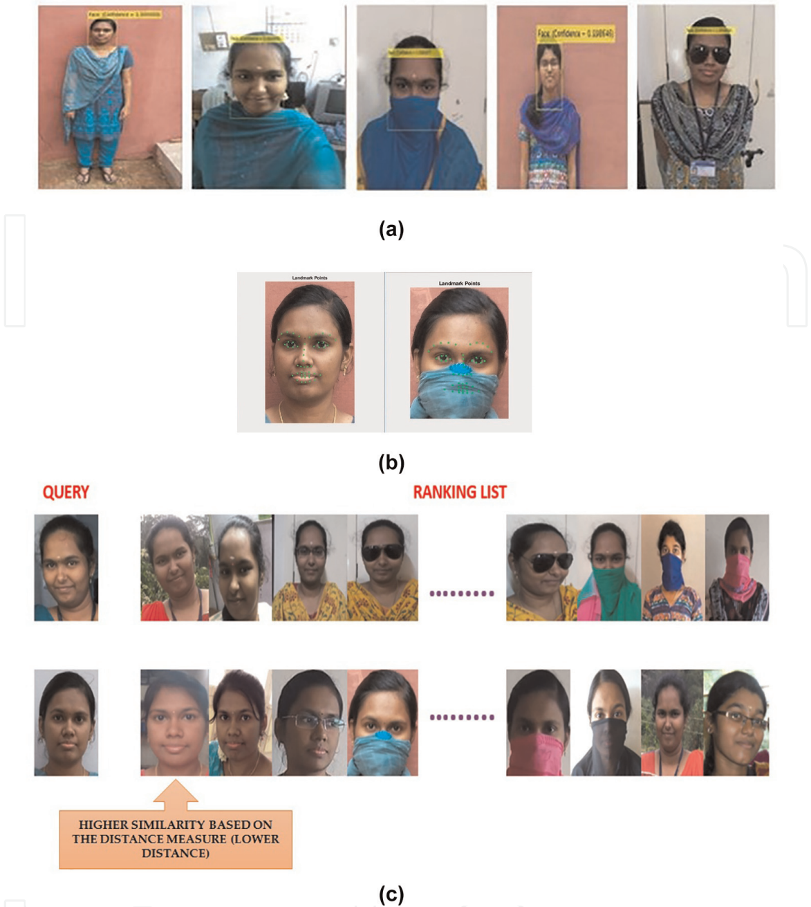
Figure 3. (a) Face detection result using R-CNN for TCE dataset, (b) detected landmark points using SDM algorithm, and (c) ranking list of the TCE gallery set with similarity.
