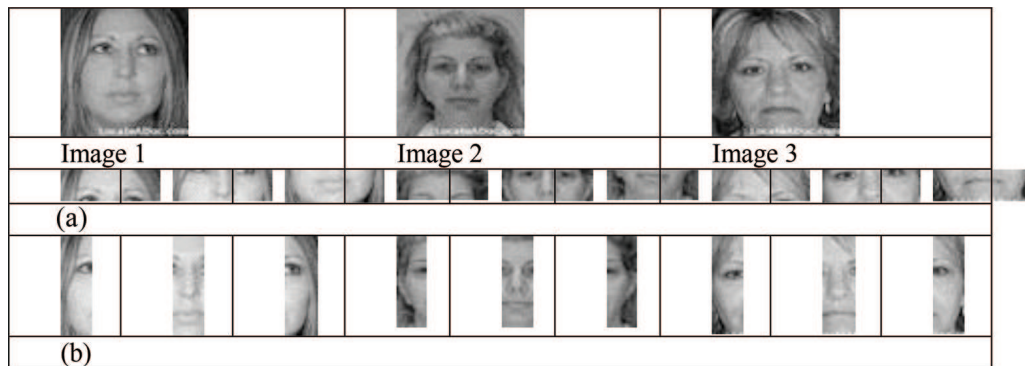
Figure 6. Computation of granular images 1, 2, and 3. (a) Horizontal granules and (b) vertical granules.
