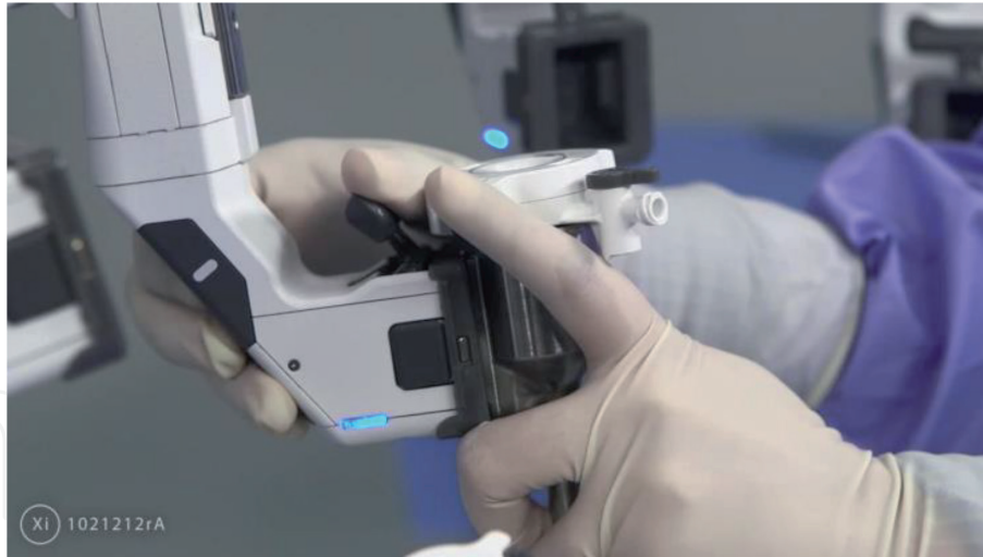
Figure 8. Docking of the robotic ports. All robotic ports require to be docked to the robot arms on the patient cart prior to their use. The metallic extension on the ports is engaged with the robot port using the port clutch in a process known as docking.
