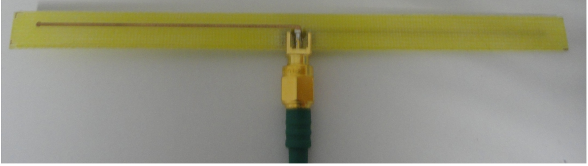
Figure 6.16: Produced dipole antenna
