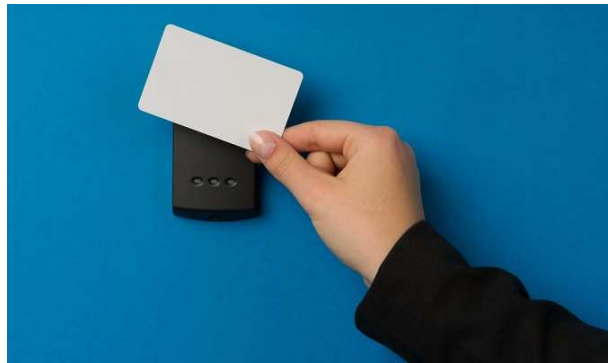
Figure 4.5: Common use of passive tags [9]
