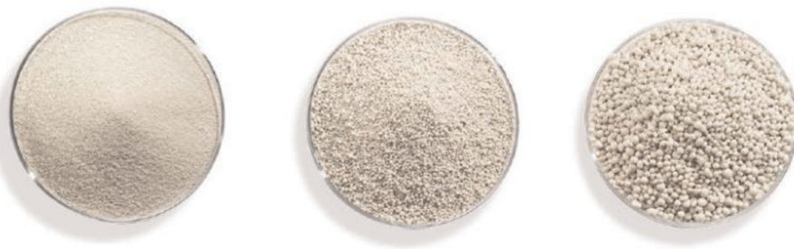
Figure 2. LWA, from left to right, Poraver 0.25–0.5, 1–2, and 2–4 mm.
