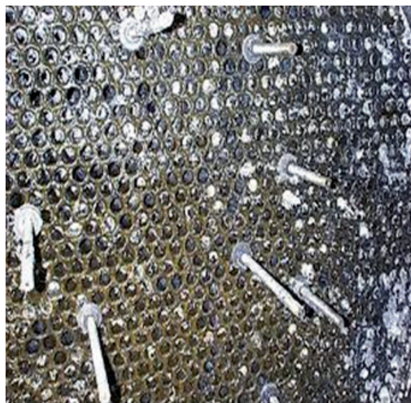
Figure 5. Icy icing of polymer products in a heat exchanger (Source: By courtesy of H&C Heat Transfer Solutions In.).
